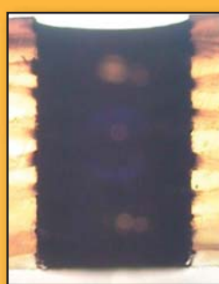
without use of hole conditioner
