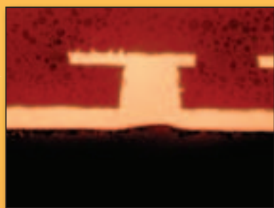
Via Diameter: 50 \mu\text{m} Via Depth: 50 \mu\text{m} Plating Thickness: 32 \mu\text{m}
