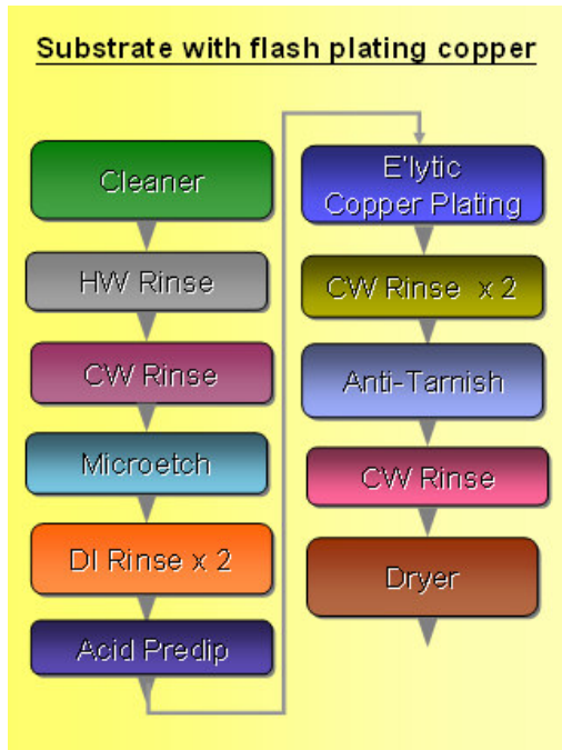
FIGURE 5. Panel Plate Process Flow
