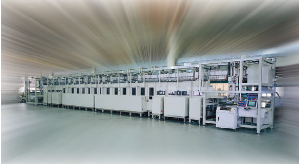
FIGURE 4. Applied Equipment Limited, VCP Vertical Copper Plater
