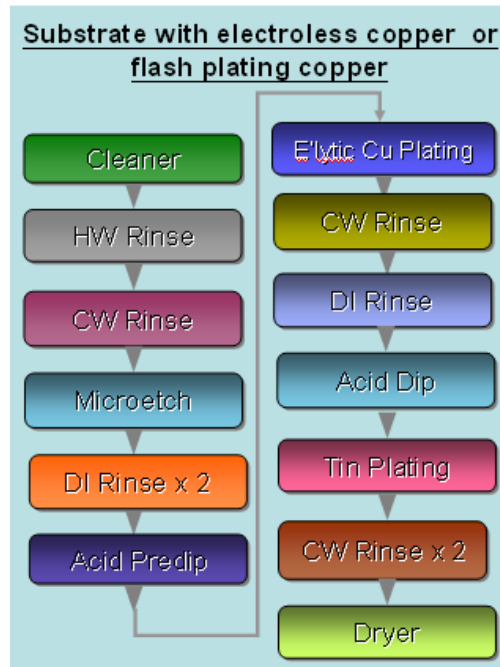
FIGURE 6. Pattern Plate Process Flow
