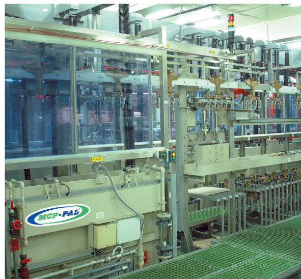
FIGURE 3. PAL, MCP-PAL™ Vertical Continuous Plating Line
