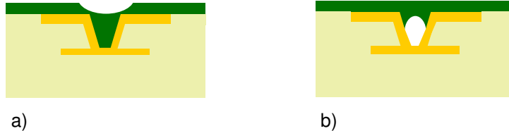
Figure 3: a) Poor solder mask coverage around blind via perimeter b) Solder mask voiding in blind via
