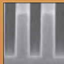
280 nm 1:1.5 Trenches at 1.3 μm FT
