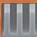
700 nm 1:1 Trenches at 3.5 μm FT
