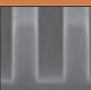
400 nm 1:1 Trenches at 1.0 μm FT
