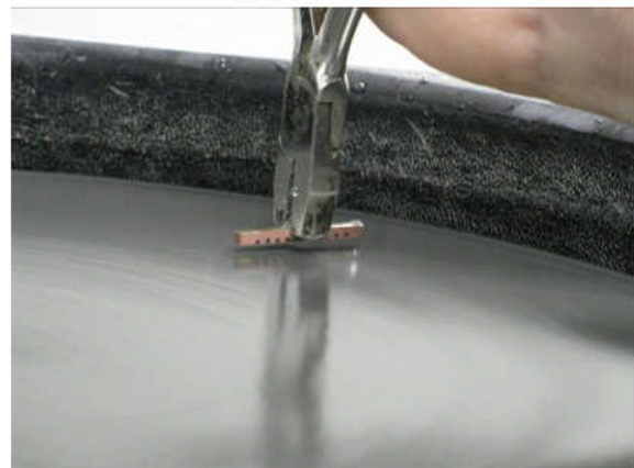
Front side rough grind
