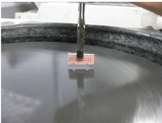
Back side rough grind
