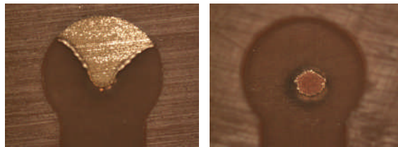
Figure 3 Peel test at via bottom after plating (Left: 3328, Right: Control)
