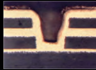
Excellent coverage in microvia 深埋孔优异的覆盖能力
