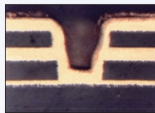
Excellent coverage in microvia 深埋孔優異的覆蓋能力
